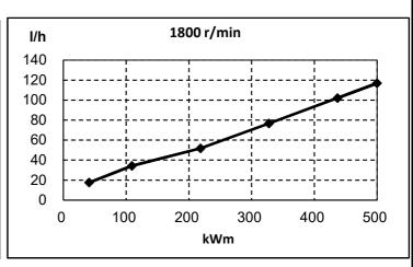
Curves shown above represent gross engine performance capabilities obtained and corrected in accordance with GB/T18297 conditions of 29.61 in Hg (100 kPa) barometric pressure [263 ft (80 m) altitude], 77 deg F (25 deg C) inlet air temperature, and 0.30 in Hg (1 kPa) water vapor pressure with No. 2 diesel fuel.
