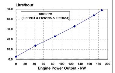
Curves shown above represent gross engine performance capabilities obtained and corrected in accordance with GB/T18297 conditions of 100kPa (29.61 in. Hg) barometric pressure [80 m (263 ft.) altitude], 25°C (77°F) inlet air temperature, and 1 kPa (0.30 in. Hg) water vapor pressure with No.0 diesel fuel. The engine may be operated without changing the fuel setting up to 2200 m (7218ft.) altitude.
