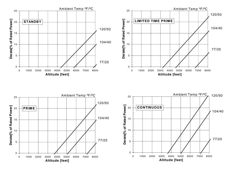
NOTE: Derates shown are based on 15 in H<sub>2</sub>0 air intake restriction and 2 in Hg exhaust back pressure.
