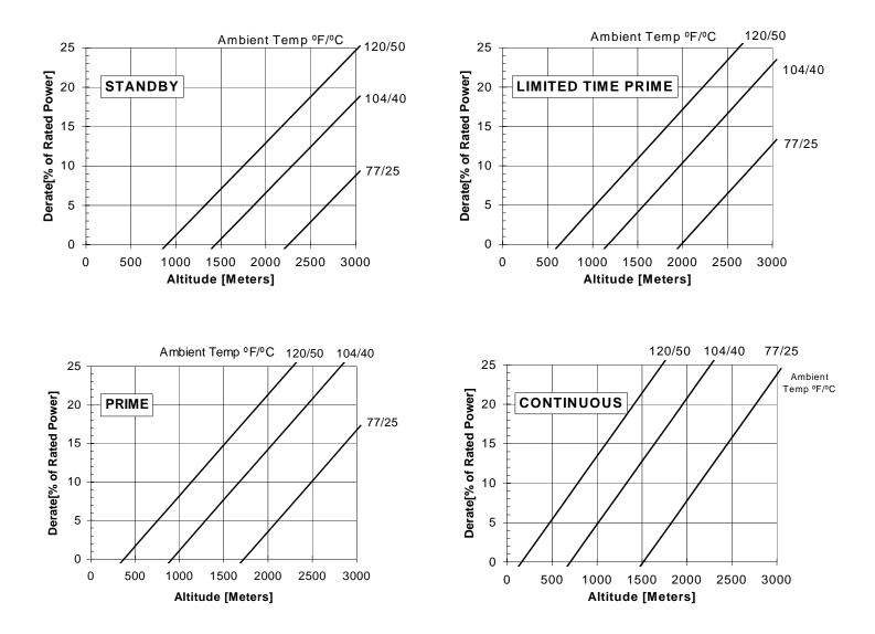
**NOTE:** Derates shown are based on 15 in  $H_20$  air intake restriction and 2 in Hg exhaust back pressure. For sustained operation above these conditions, derate by an additional 5% per 1000 ft (300 m) and 9% per 18° F (10° C).
